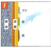
Remove mud, moss, bird dropping etc. from the coated surface. A clean surface it essential for the release agent to penetrate.
