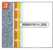
Determine the time to let the release agent to gradually penetrate into the coating film.
