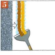
When peeled off with a scraper, it can often come off in a long sheet.
