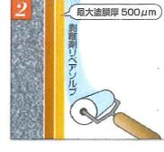
Apply a coating using a spray gun, roller or a brush.
